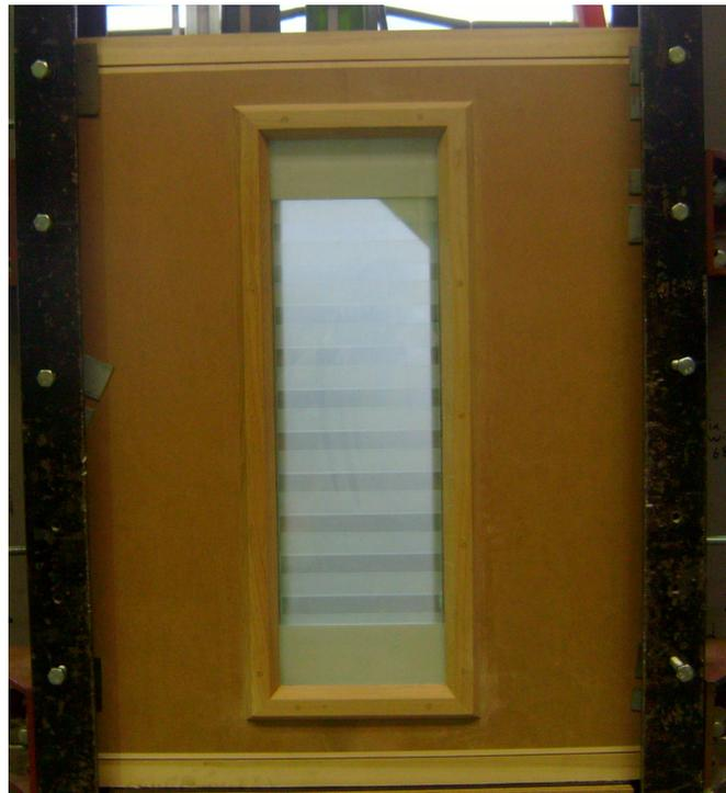
Figure 1 View of Vision panel from impact face prior to testing
