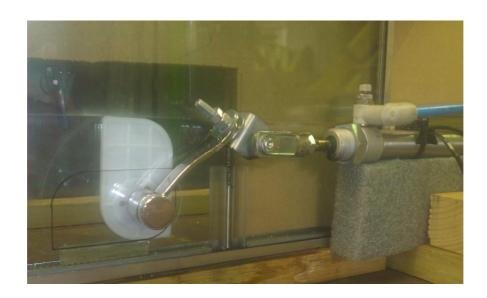
The operating force of the handle was measured at regular intervals of testing. The pneumatic controller was set up to open and close the panel by pushing and pulling the handle continuously and the number of cycles recorded. The mechanism was inspected at regular intervals to check for signs of wear and tear and also the functionality of the system.
